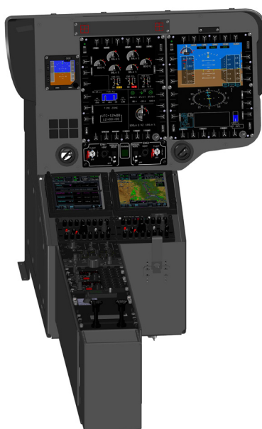
Figure 1.7: Example of standard single pilot instrument panel with two MFD
