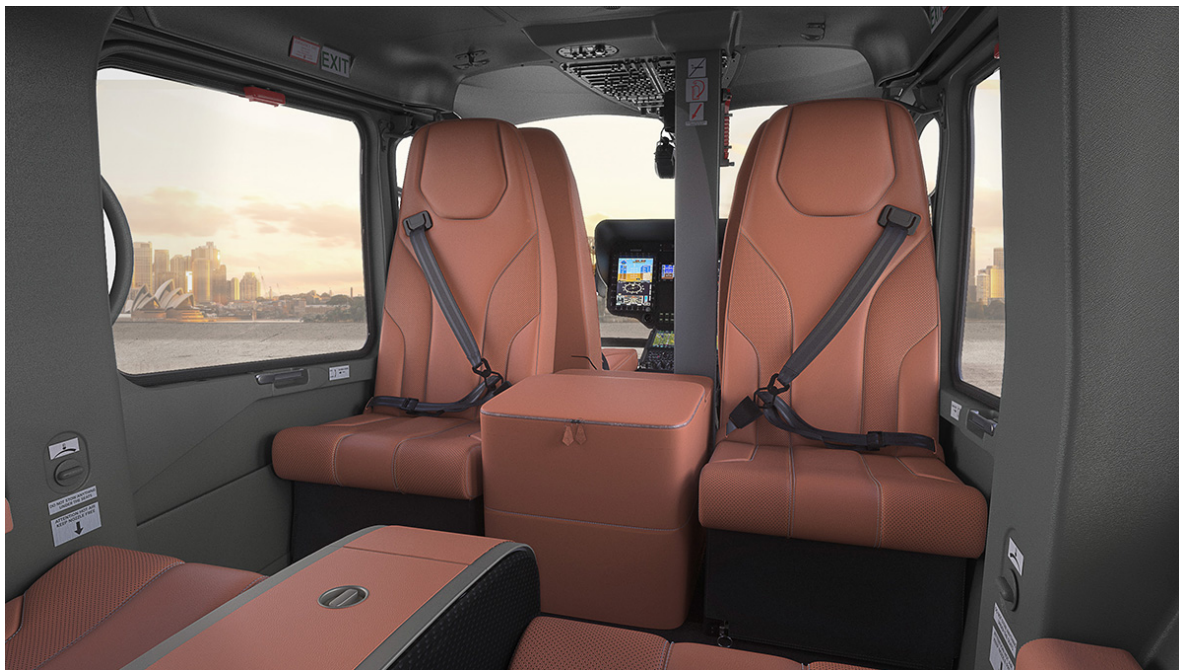
Figure 4.6: Example of ACH Line, 4 passenger solution with one cabinet and one multifunctional box
