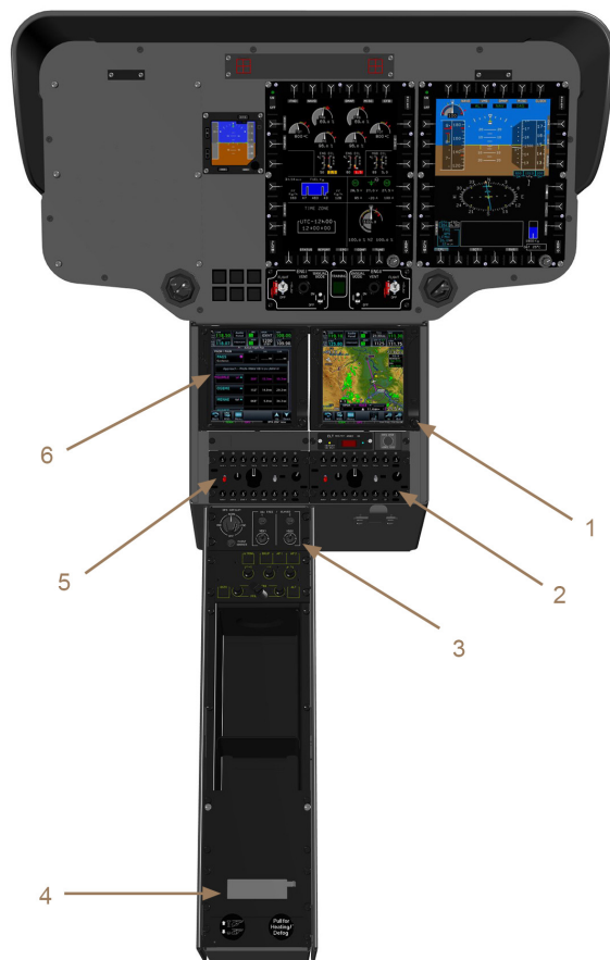
Figure 5.2: Avionics layout Single Pilot IFR GTN 750Xi (Garmin)
