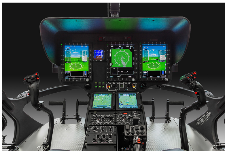
Figure 1.3: Typical instrument panel
