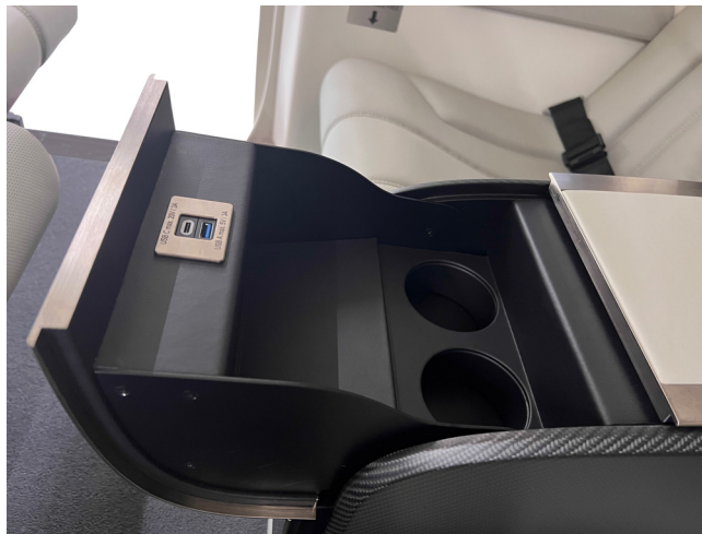
Figure 1.12: Example of ACH Line rear cabinet with USB type A and C sockets
