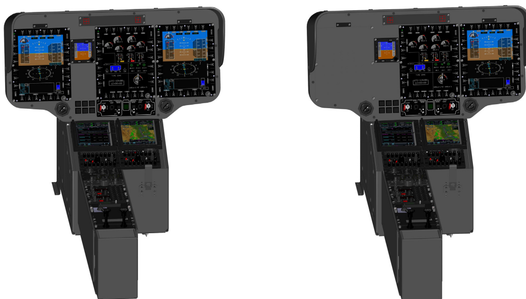
Figure 1.6: Example of extended instrument panel with three (LH) and with two (RH) Multifunctional displays
